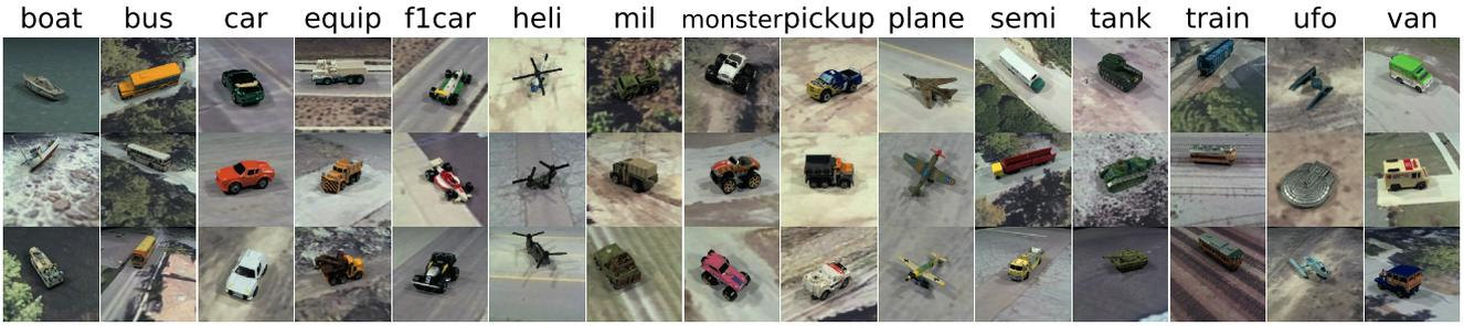
**Figure 2:** The iLab-20M dataset provides toy vehicle images from 15 categories in various viewpoints, lighting conditions, and backgrounds. Cropped images of sample object instances for each category are shown above. Sample images demonstrate rich intra-class variations in shape, size, color, and texture.
